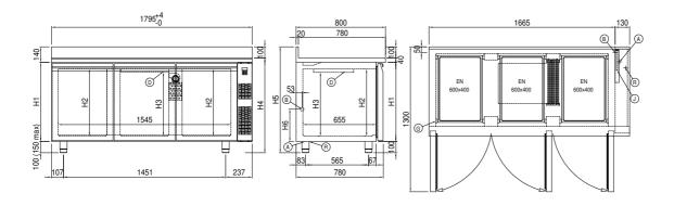
A: Power supply cable outlet B: Condensation water drain D: Airflow conveyor
