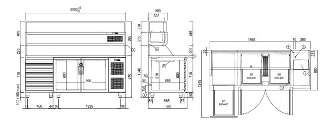
A: Power supply cable outlet B: Condensation water drain D: Airflow conveyor
