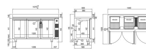
A: Power supply cable outlet B: Condensation water drain D: Airflow conveyor
