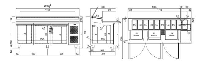
A: Power supply cable outlet B: Condensation water drain D: Airflow conveyor
