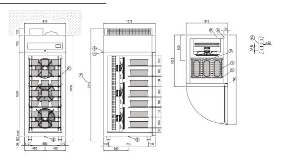
A: Power supply cable outlet B: Condensation water drain G: Racks pitch
