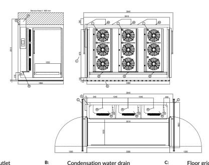
A: Power supply cable outlet B: Condensation water drain Floor grid for condensate drainage (recommended)
