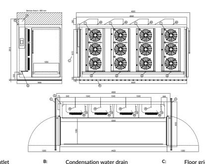
A: Power supply cable outlet B: Condensation water drain Floor grid for condensate drainage (recommended)
